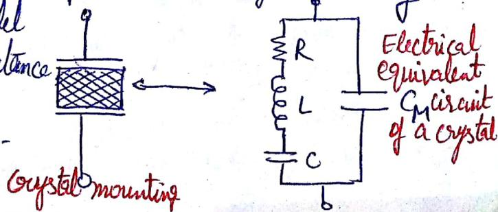
Because of presence of  $C_m$ , the crystal has two resonant frequencies. One of these is the series resonant frequency  $f_s$  at which  $2\pi fL = \frac{1}{2\pi fC}$  and in this case the crystal impedance is very low. The other is parallel resonance frequency  $f_p$  which is due to parallel resonance of capacitance  $C_m$  and the reactance of the series circuit. In this case crystal impedance is very high.
