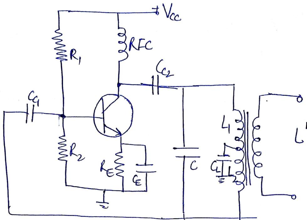
Ex In a Hartley oscillator, the tank circuit has the capacitance of  $100\text{ pF}$ . The value of inductance between the collector and tapping point is  $30\text{ mH}$  and the value of inductance between the tapping point and the transistor base is  $1 \times 10^{-8}\text{ H}$ . Determine the frequency of oscillations. Neglect the mutual inductance.
