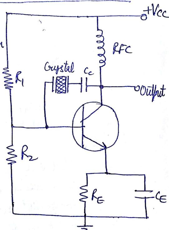
The coupling capacitor  $C_c$  has negligible impedance at the circuit operating frequency but blocks any dc between collector and base. The circuit is called the Pierce Crystal. Variations in supply voltage, transistor parameters, etc. have no effect on the circuit operating frequency which is held stabilized by the crystal.
