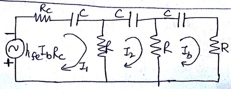
Making above ~~of~~ assumptions and replacing current source by equivalent voltage source, the simplified equivalent circuit is shown in figure (b)
