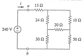
Q.3(a) For the circuit given below, calculate the current, voltage and power associated with the [2] CO1 BL3  $20k\Omega$  resistor.
