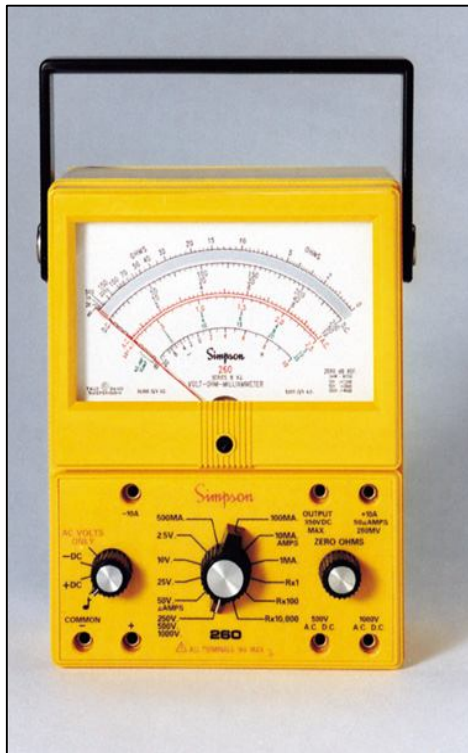
Analog VOM that combines a function selector and range switch.
